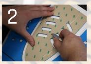
Using a knife, score the reverse of the centre section of your pad pad along the 3M backing between any cut outs on your design. Cut through the 3M backing only, not into the foam.
